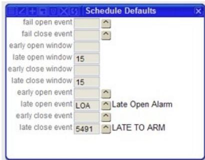
The standard Open and Close [Event Codes](#) should be set as log only. Alarms are generated by separate events codes that can drive [Action Plans](#). Fail Open/Close Event can be set to generate a specific event code when an open or close does not occur as scheduled. Alternatively, Early Open, Late Open, Early Close, and Late Close Events will occur when an open or close comes in outside the normal schedule.
